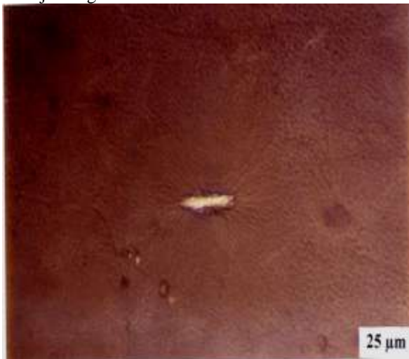
Fig. 4. Optical photograph of isolated single lamella of isotactic polypropylene which crystallized at T_c = 125^{\circ}\text{C} .
